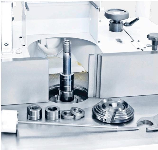
SK40 cutter arbour clamping system
