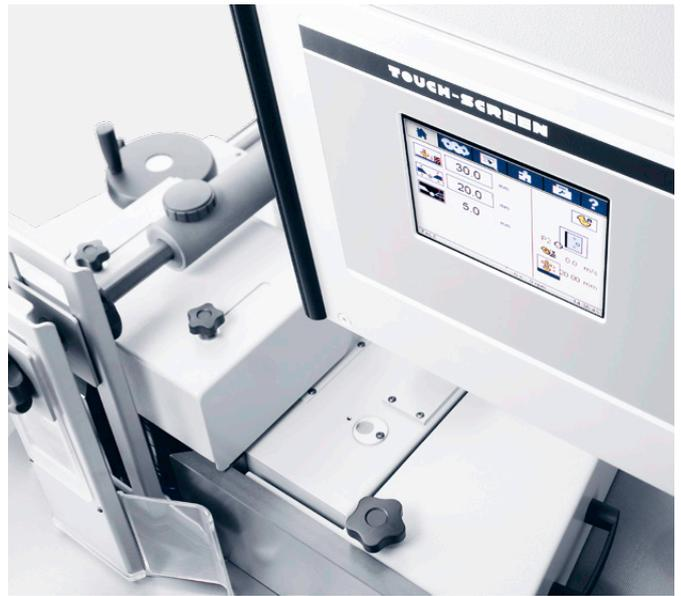
Digital display of the position of the fence jaw (right)
