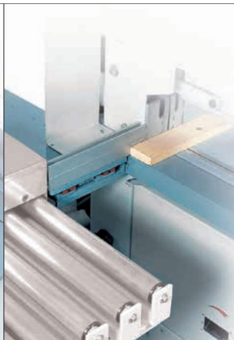
Trap door for expelling trimmed material from headpiece and scraps from straight cut tailpiece (open)
