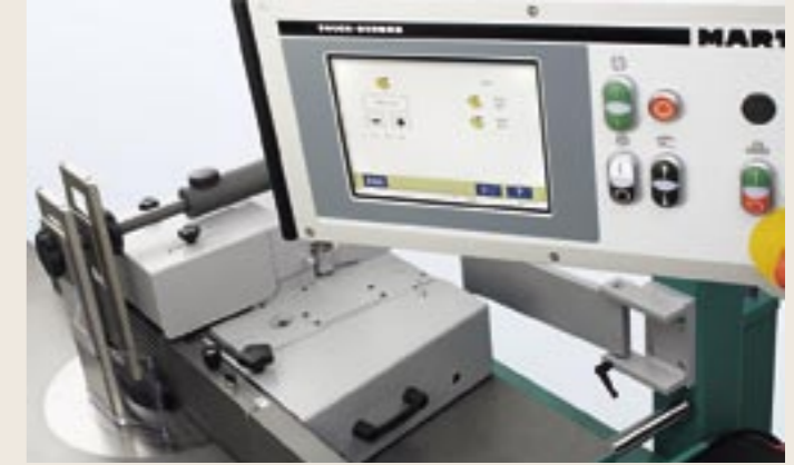
Variable speed inverter control
