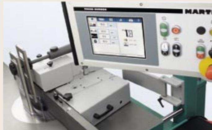
Motorized positioning of the infeed fence jaw
