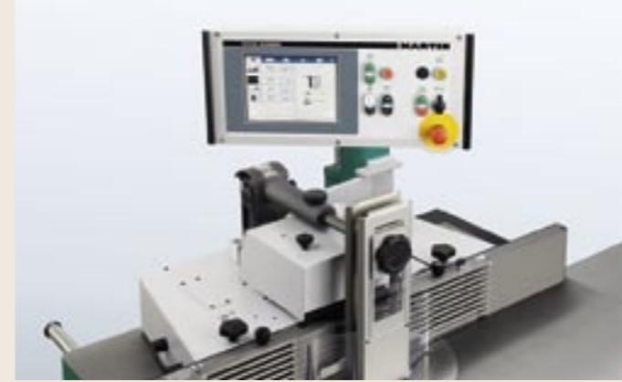
Electronic fence positioning
