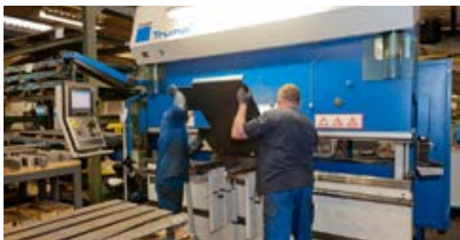
Computer assisted steel plate bending
