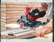
Thanks to the generously-sized angle scale and precise double clamp, miter cuts can be realized that ensure a perfect fit - as illustrated here on exterior cladding.
