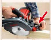
The pivoting guard is retracted quickly and easily by means of a lever for convenience and safety when executing bevel and plunge cuts. With the compact and ultra-performing K 65 cc, you can achieve superb quality cuts at depths of up to 67 millimeters - and this from a portable circular saw with the best power-to-weight ratio in its class. It offers all the weight and handling advantages of a 55-series machine with the cutting depth of a 65 mm model.
