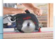
Dispensing with a detachable riving knife, the FLIPPKEIL permits reliable, convenient and straightforward plunge cutting.
