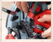
The K 65 cc's cutting depth can be preset and locked in the range from 8 to 67 mm.
