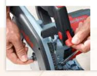
To change blades, the K 65 cc sawblade is locked simply by pressing a button, which automatically engages the starting lockout. The sawblade can then be changed quickly and easily using the Allen key attached to the machine.
