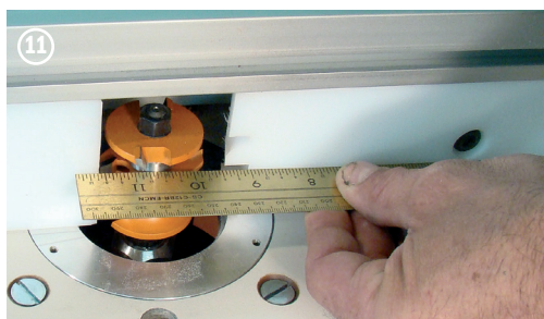
11. Set the fence by bridging the opening in the fence with a straight edge. The straight edge should touch both faces of the fence and the ball bearing on the router bit. You won't be using the miter gauge, so it's not important to make the fence parallel to the miter gauge slot for these cuts.
