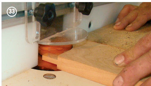
33. Make a test cut. Use a piece of scrap behind the rail to prevent blowout when the bit exits. Narrow pieces must be clamped into a miter gauge. Check the fit of the tenon. If it's too loose add spacers between the upper and lower cutter sets. If the tenon is too tight remove spacers. Make test cuts until you've achieved a perfect fit.
