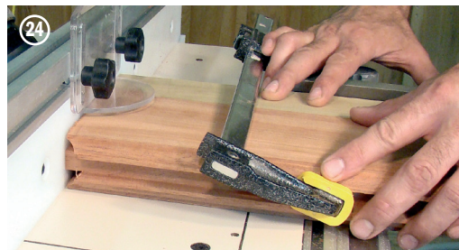
24. Clamp the square edge of the support block against the material when the trailing edge is square. Machine both ends of all the rails.
