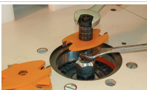
Tighten the bit stack.
