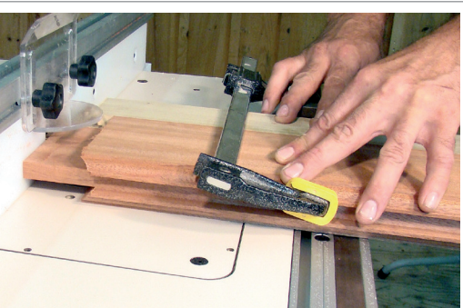
25. Cut the extra-long tenons by moving the fence back from the cutter and undercutting the tenon produced in the previous steps.
