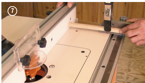
7. As before, use the Gauge Stick to set the fence parallel to the miter gauge slot.
