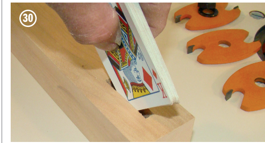
30. Find the size of the tenon you need to produce. An easy way to do this is by slipping a stack of playing cards in to the mortise (or groove if you're making a passage door) to gauge the size.
