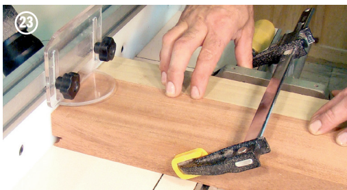
23. Use the support block on the trailing edge of the cut to eliminate chipping when coping the end grain of the rails.
