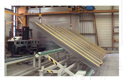
→ Optionally the working table can be supplied with a tilting option to allow the element to be lifted off with a vertical crane
