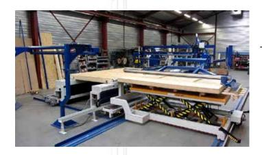
A range of optional stud / joist feeding carriages are available to supply the materials in a convenient location for the operator
