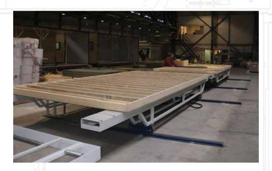
→ One fixed table and one moveable table on guide rails with manual locking arrangement
