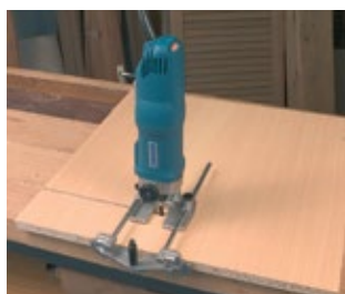
Trimming parallel slots.
