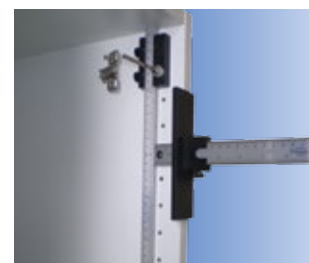
Drilling for placing invisible hinges.
