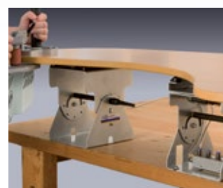
Gripping large pieces with the help of an SVN470 auxiliary unit.
