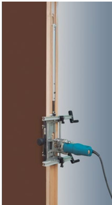
Making the second recess on the frame.
