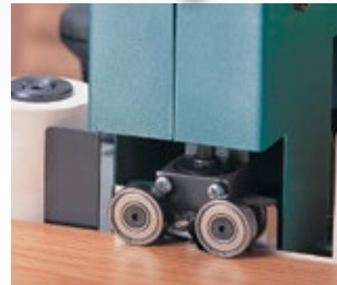
Power trimming unit: trimming both sides simultaneously.
