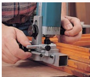
Slotting a window, flashing side.
