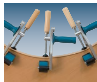
Fixing tapes on concave panels
