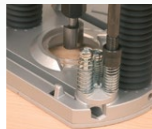
Quick adjustment of routing depth with 3 positions.
