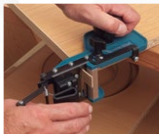
Cutting on both sides on straight panels.
