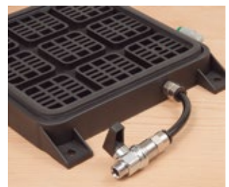
Includes quick connection tube to the electric clamping system SVE600 (optional).
