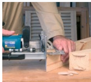
Stronger joints with No. 6 splines.
