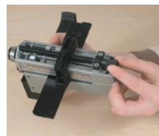
Micrometric regulation of the cutting width.
