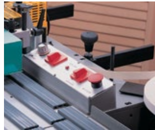
Safety control (STOP). Electronic temperature control.
